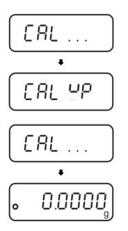
When the adjustment is successfully completed, you will see the <CAL up> indication.
