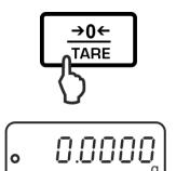
Unload the balance. Press the **TARE** key.
