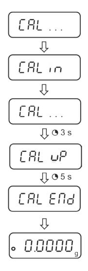
In case of the adjustment error (e.g. object on the plate) the following error message will be displayed: <CAL NO>, repeat the adjustment procedure.
